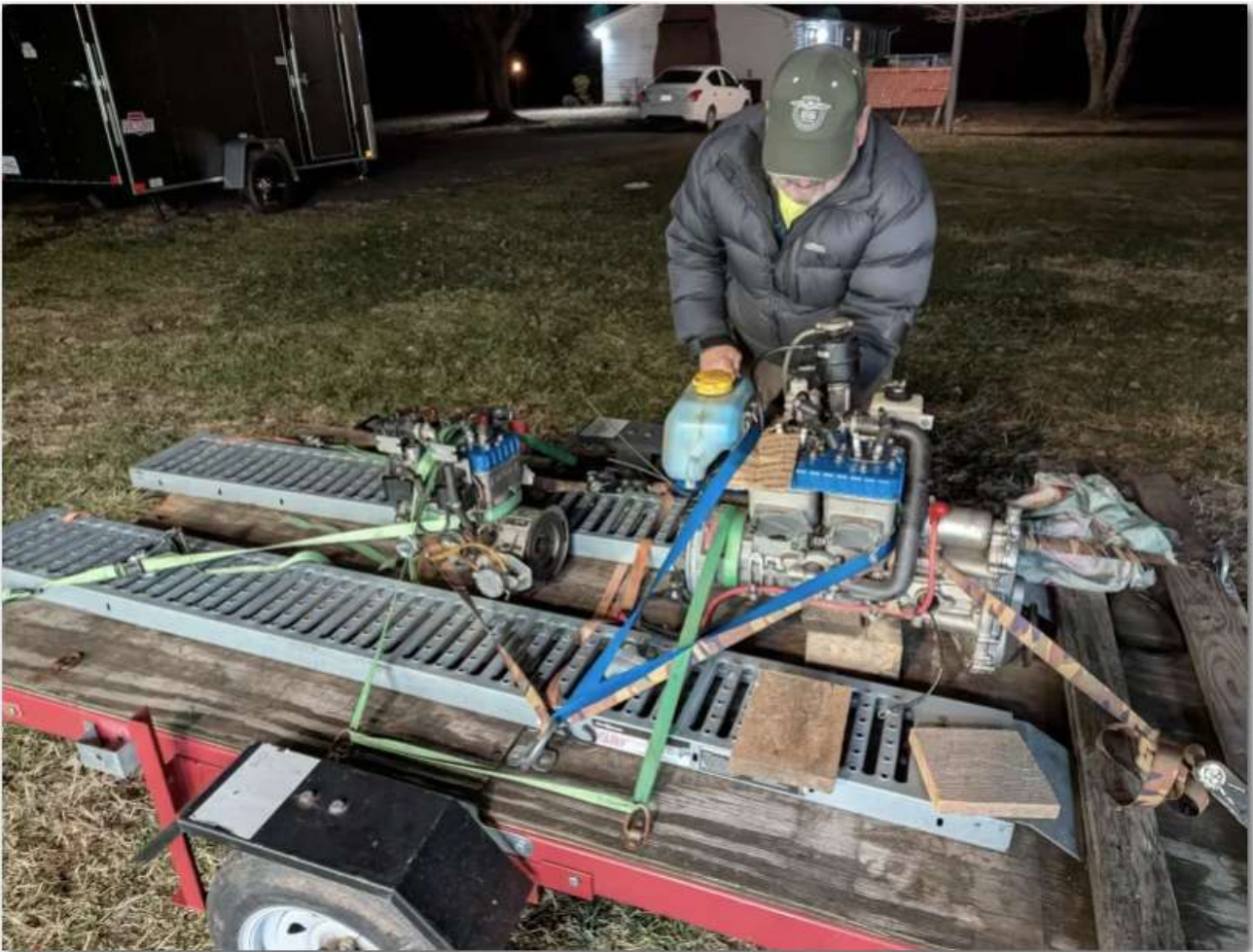
Michael Bishton takes two Rotax 582s – one from the Challenger kit and one from the Breese –off to be inspected in Pennsylvania
