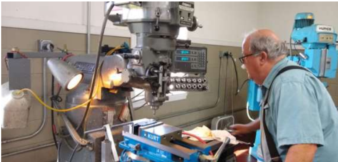
Guided by the blue position digits, Luther moves the cutting head
