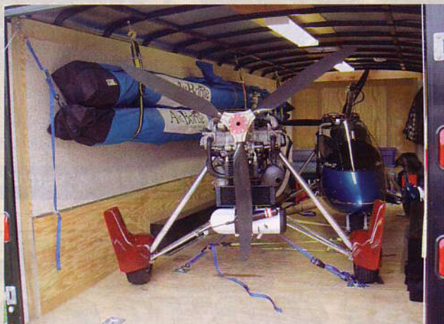
Our car trailer converted to an airplane trailer has an inside length of 20 feet to accommodate the 19-foot long trike wings. It can hold three trikes in a pinch. It was our hangar-on-wheels, accommodating our aircraft and their associated gear.
