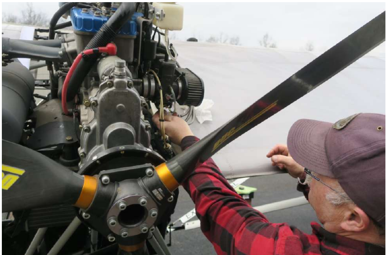
Tim removes a fuel filter from one of the carburetors
