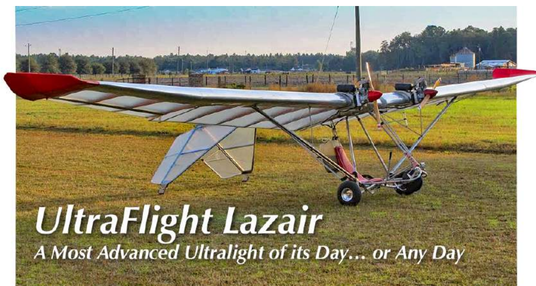
The Lazair. Bob's early model had 11hp, taking both engines together.
