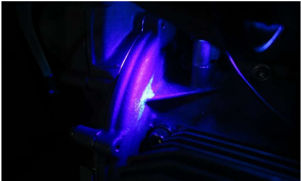
The leak under ultraviolet light
