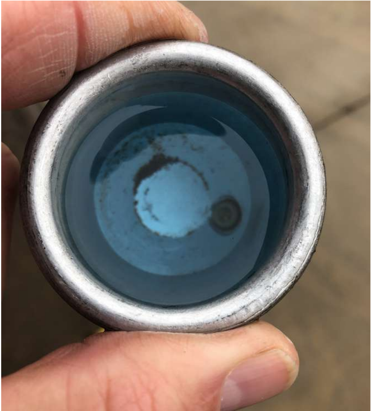
Fuel system debris in the gascolator
