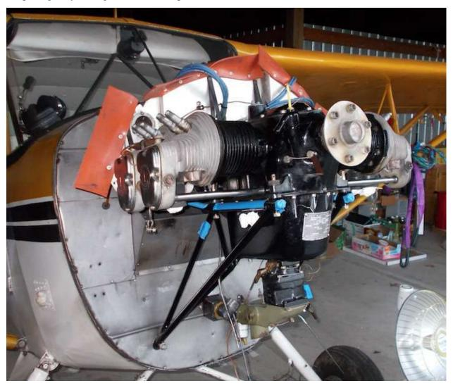
You would think that, with the new engine bolted in place, that you are close to the end of the engine installation – Not so!
