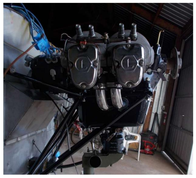
Although the carburetors on both engines were the same, the metal boxes bolted underneath are airframe specific – Switching these metal boxes was the next step.
