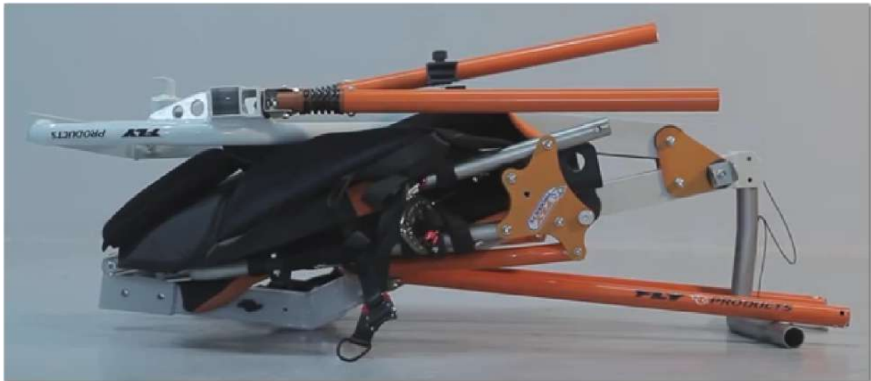
Folded Vertigo PPG trike. See it being folded in this demonstration video
