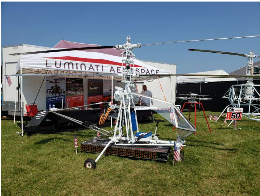
Luminati Aerospace's electric helicopter with counter-rotating rotors
