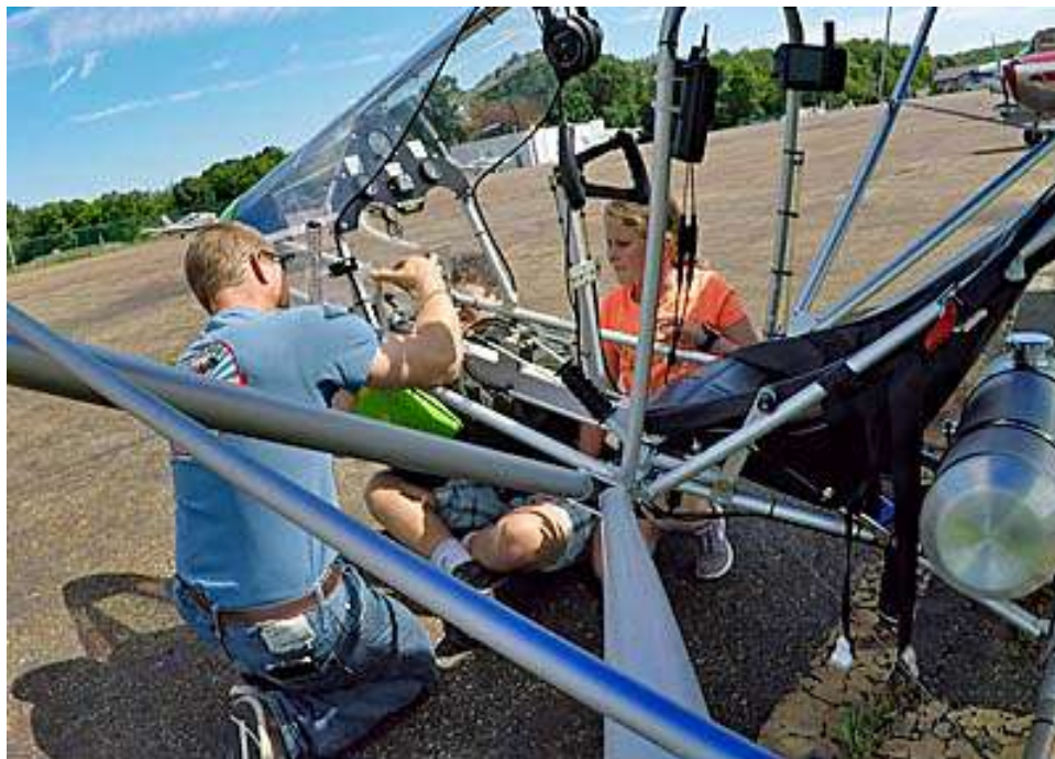
Minor repair to nosewheel steering linkage shows this is a family affair
