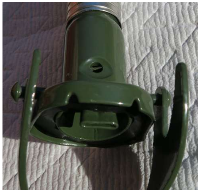
Detail showing vent tube inside spout. Air comes from the hole outside the cap.
