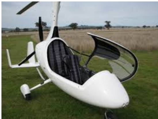
Enclosed, tandem seating: AutoGyro Calidus
