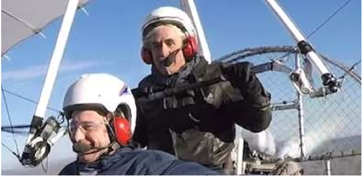
Birdman Moullec's control bar - with swiveling offset
