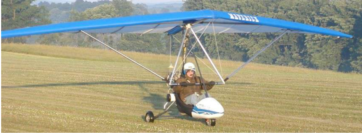
Normal position of a trike control bar, rigidly attached to the wing
