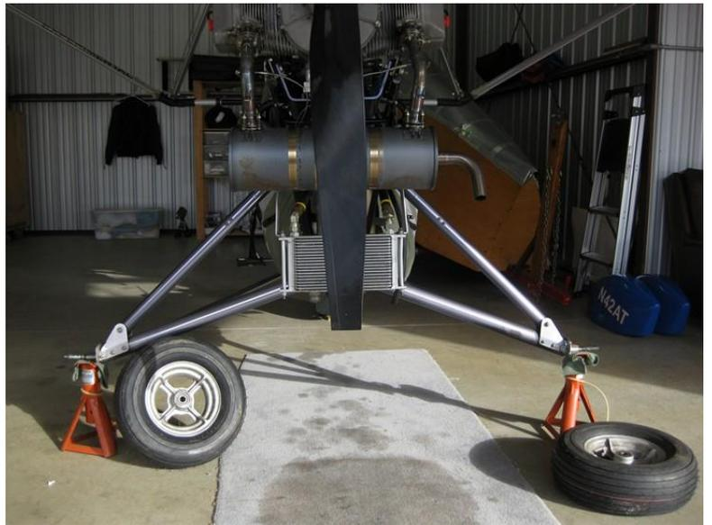
Two tires mounted on the wheels cost \$96. It took me about an hour to remove the fairings and wheels, an hour to replace them. Because I fly off concrete, I got only 74 hours out of the last pair of mains, which is a lot less than I would like. (The nose wheel lasts forever.) I inflate them to 18psi. The trike, empty, weighs 485 pounds. If any of you has a better system, I am definitely open to suggestions.
