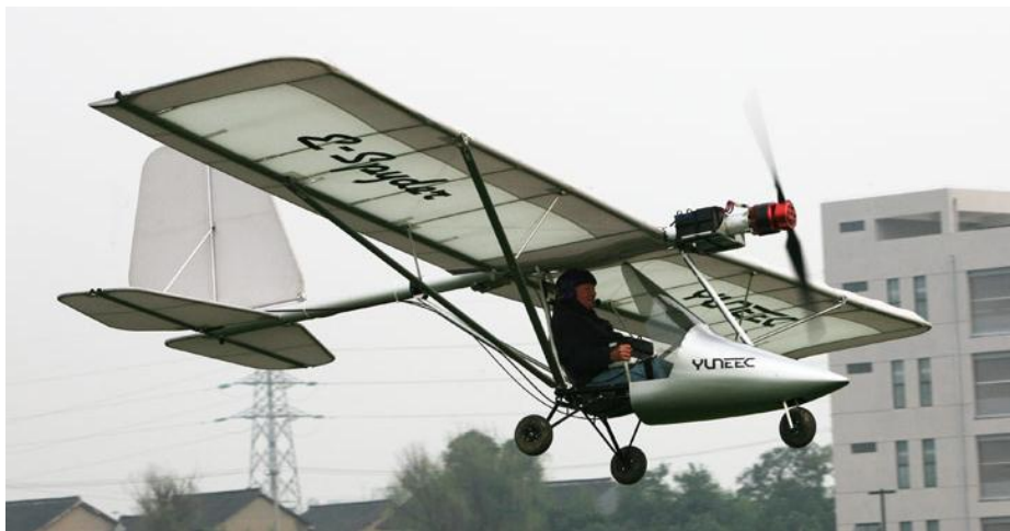
Yuneec e-Spyder. 27hp motor, 37mph cruise, 1 hour duration, 253 lbs.
