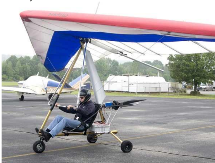
ElectraFlyer. 18hp, 25mph cruise, 2 hour duration, 247 lbs.
